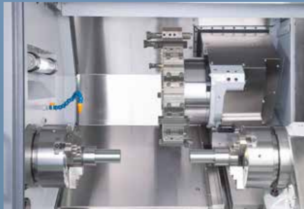
Two Spindle Single Turret (Hydraulic/Servo)
