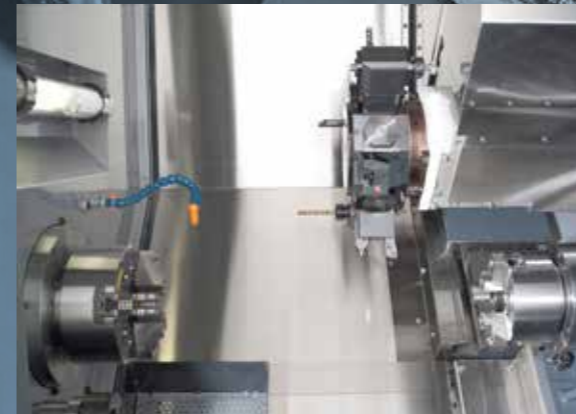
Two Spindle Single Turret (Power turret + Y-axis)
